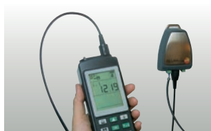
Inspection of transmitters with 4 to 20 mA interface
