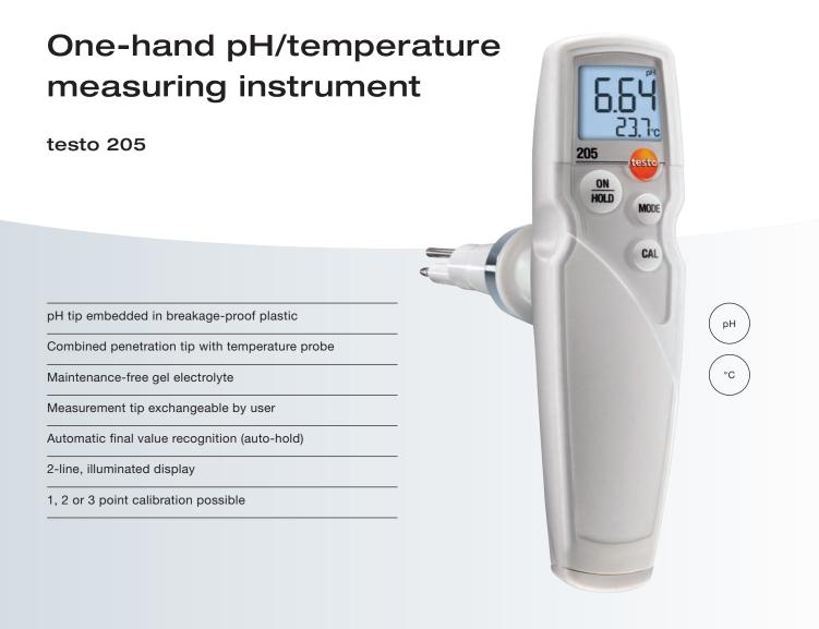
The testo 205 is a robust food penetration measuring instrument for temperature and pH values, with automatic temperature compensation. The robust penetration measurement tip is exchangeable and insenstitive to dirt thanks to the hole diaphragm. The instrument is especially well suited to pH measurements in semi-solid media such as meat. The storage cap filled with electrolyte gel is used for storing the probe between measurements.
