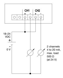
Connection plan 4-wire technology (0 to 20 mA / 4 to 20 mA / 0 to 1 V / 0 to 5 V / 0 to 10 V)
