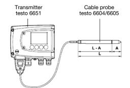
L = Probe length L-A = Probe length – length protective cal A = 35 mm
