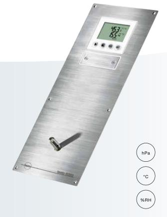
The differential pressure transmitter testo 6383 was developed specially for monitoring low differential pressures in the measuring range from 10 Pa to 10 hPa. In cleanroom technology, the maintenance of positive pressure prevents the entry of contaminated air in critical zones. Thanks to an optional internal or external probe from the probe series 6610, the additional recording of humidity and temperature with one instrument is also possible.
